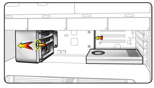
Note: Some graphics cards require 1 or 2 booster cables connecting card to auxiliary power connectors on backplane board. If your card has booster cables, disconnect them from backplane board.
